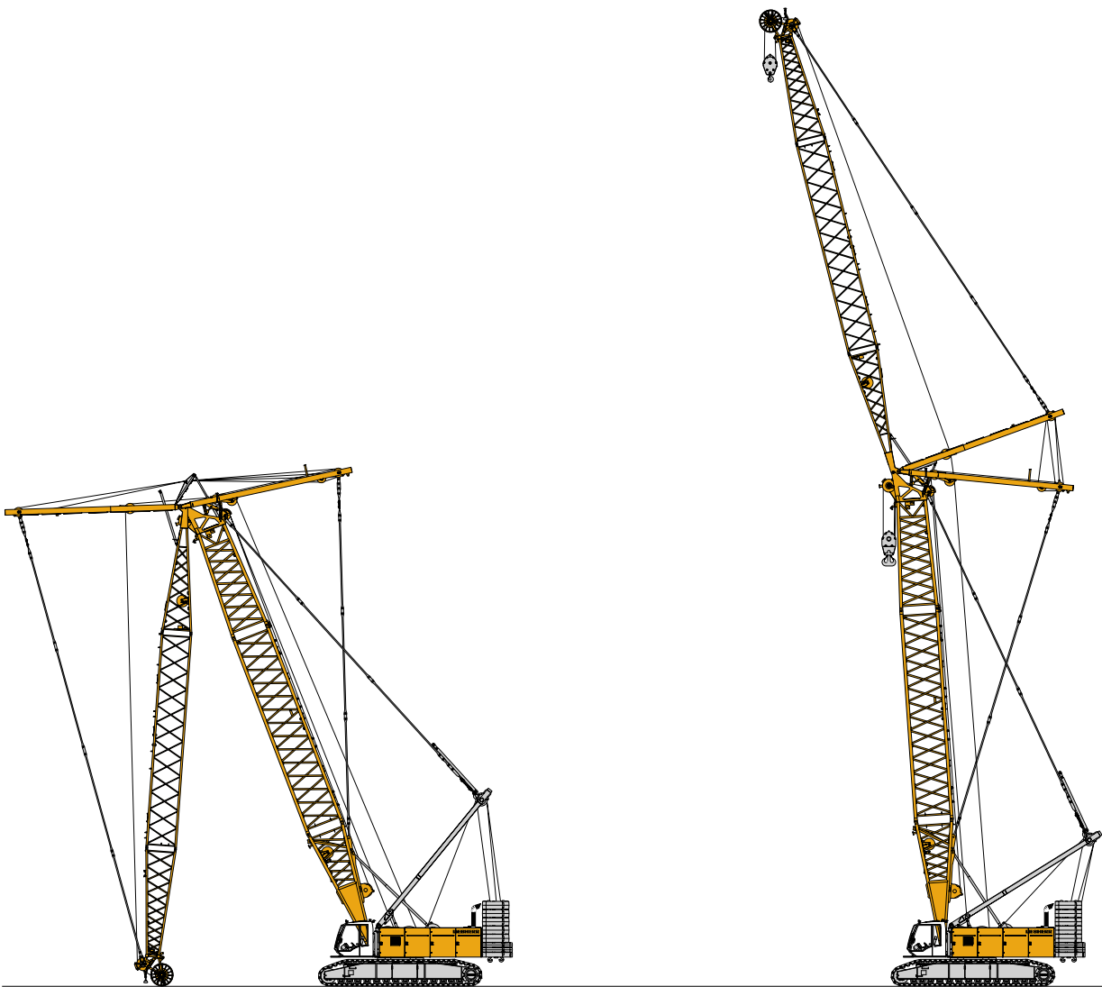
Erecting of main boom and luffing jib
